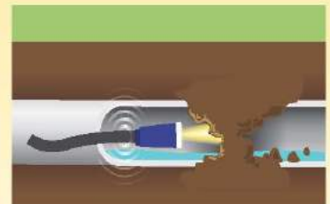
A CRUSHED PIPE with a camera showing it's location.
