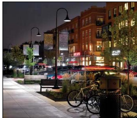
This photo shows pedestrian-scaled lighting which is low enough to the ground to illuminate walkways and the faces of pedestrians.
