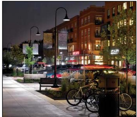
This photo shows pedestrian-scaled lighting which is low enough to the ground to illuminate walkways and the faces of pedestrians. Photo credit: SFMTA, 2013.
